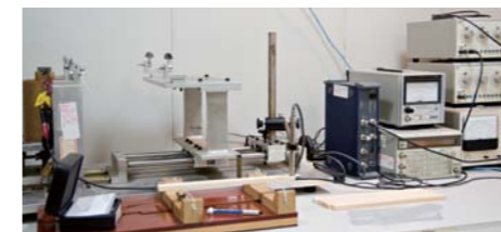
FFT analysis is used to acquire data on the sonic properties of various finishes.
