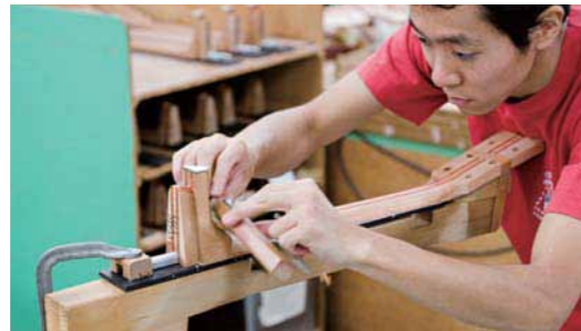
Refining body contour on a purpose-built belt sander.
