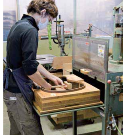
A craftsman loads a body assembly into the contouring sander.
