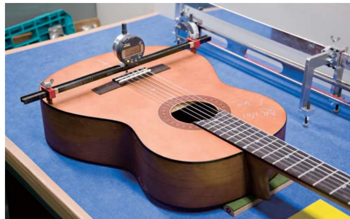
Test guitars are carefully measured for warpage and distortion as they are moved from one extreme environment to another.
