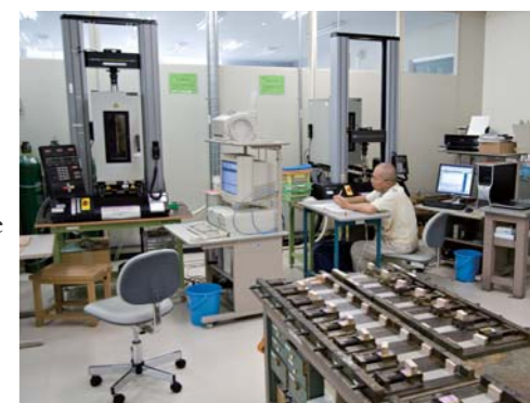
This area of the research center is devoted to testing the characteristics of wood adhesives.
