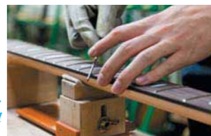
Properly leveled frets are essential for optimum playability.
