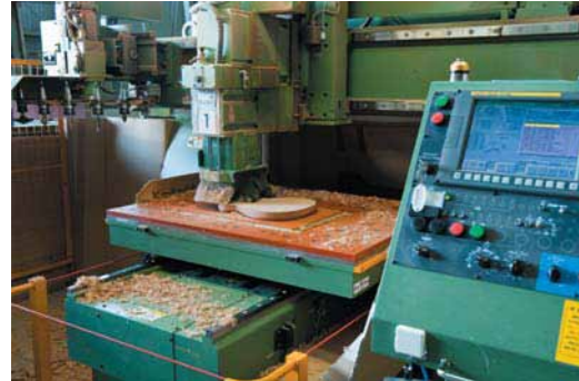
Solid electric guitar and bass bodies are initially cut and shaped on computer controlled milling machines.
