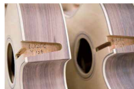
Bodies numbered so they can be reunited with perfectly matched necks after finishing.
