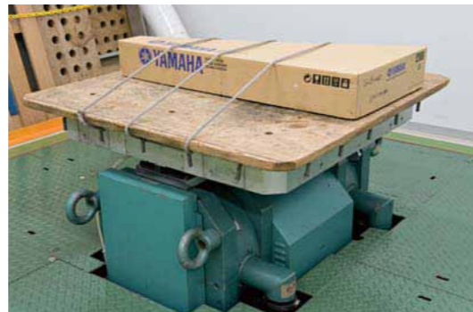
Vibration table testing simulates the type of vibration products are likely to encounter during transportation.
