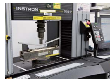
Guitar truss rods being tested under tons of pressure at Yamaha’s certified Quality Support Center.
