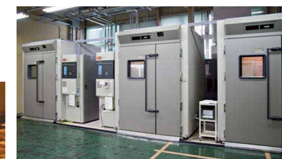
Some of the temperature and humidity testing chambers used for accelerated environmental testing of guitars.
