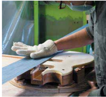
Refining body contour on a purpose-built belt sander.
