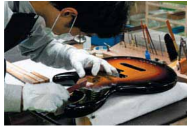
Fine tuning the neck recess in a BB-series bass body.
