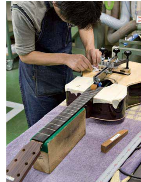
Special tools assist in precise positioning of critical parts and ensure consistent assembly quality.
