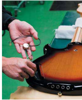
Installing the wiring and controls in a BB-series bass.
