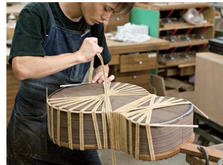
It may look easy, but guitar binding is extremely difficult to apply properly and consistently.
